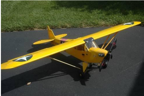
Great Planes Cub ARF. 80ö WS. Glow powered w McDaniels glow driver
